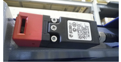
Safety guards prevent access to machine while machine is operating.
