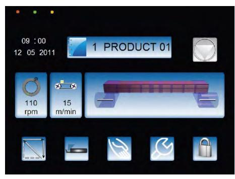
The new 7-inch, 65,000 colour touch screen provides complete control of all processes with the touch of a finger. Accurate, easy to understand controls are displayed on every screen allowing for quick and simple operation. Store up to 20 unique, user-defined wrapping programs.
