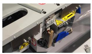
Automatic clamp, cut and seal unit neatly cuts the film after wrapping and seals the film tail to the product.
