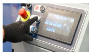
Intuitive 7" color touchscreen control panel provides quick and easy access to machine operation. Up to 20 custom programs can be stored and recalled.
