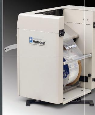
Open load area and controlled seal bar maximize loading flexibility and operator safety
