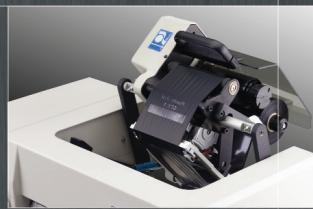
Turntable design enables easy access to bags, while the AutoThread™ feature simplifies bag changeovers
